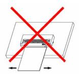
3) Due to the structure of the connectors, they do not have string resistance to upward pulling; therefore, support the FPC/FFC when a pulling force is applied to it.
